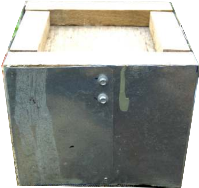
Top View of Cover before gluing tile and filling with Foam
